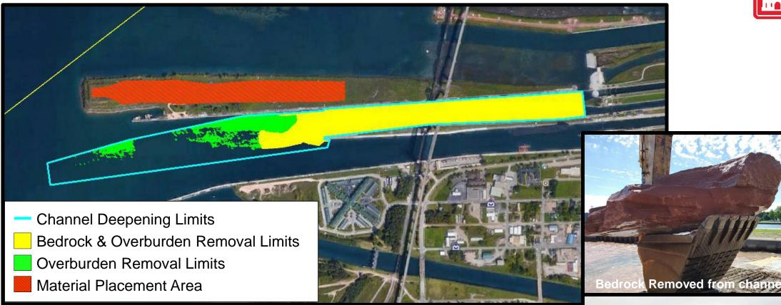
**Scope**: Remove 250,000 CY of Jacobsville sandstone and overburden to deepen the Upstream Approach Channel to depth of 30 feet **Construction Status**:
