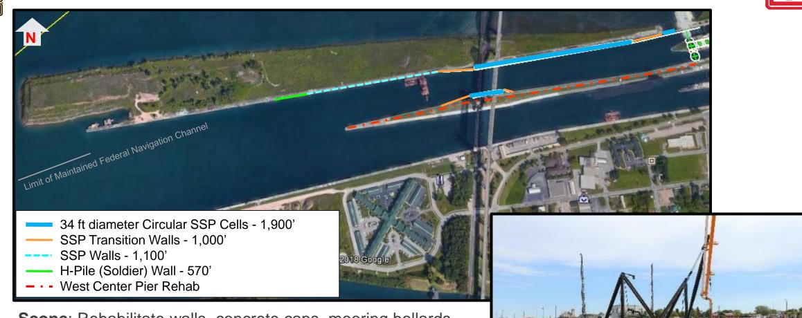
**Scope**: Rehabilitate walls, concrete caps, mooring bollards, electrical, and lighting upstream of the New Soo Lock **Project Status**:
